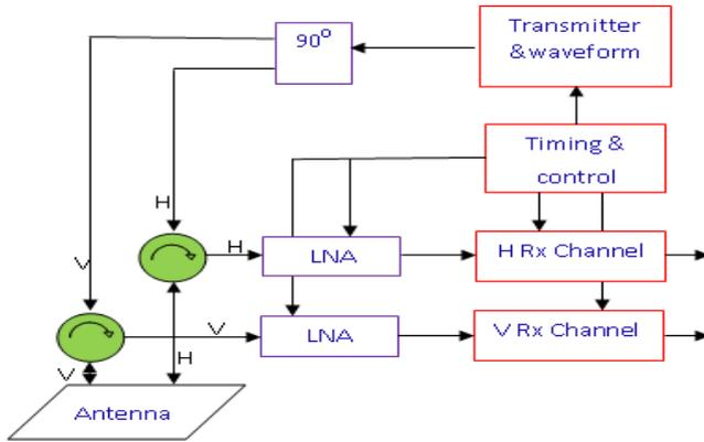
**Fig 1: Hybrid polarity SAR architecture of RISAT-1**
